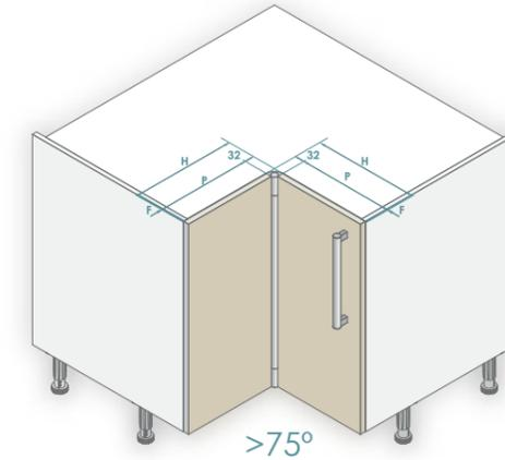
Compact takes up 32 mm in 90° corners, independently of the thickness of doors. It functions perfectly for corners >75°
